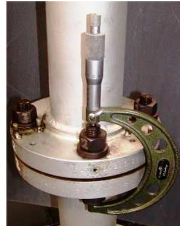
**FIGURE 5: BOLT ELONGATION MEASUREMENT**
