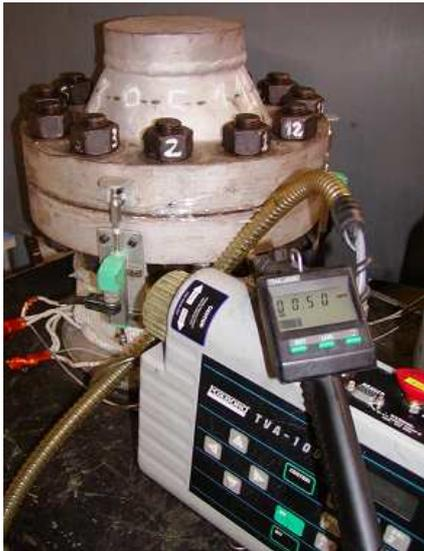
**FIGURE 3: 6 in – CLASS 900 TEST RIG**
