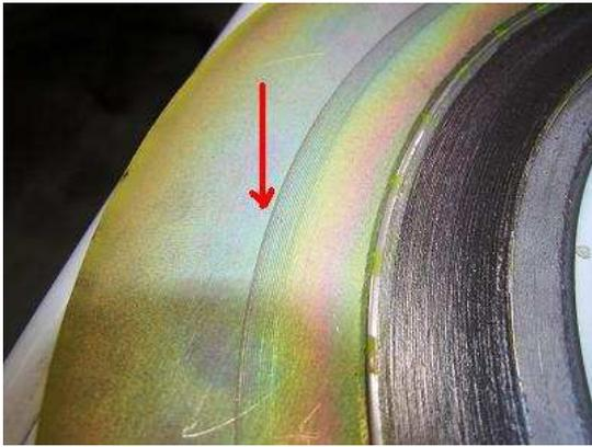
FIGURE 15: RAISED FACE GUIDE RING CONTACT
